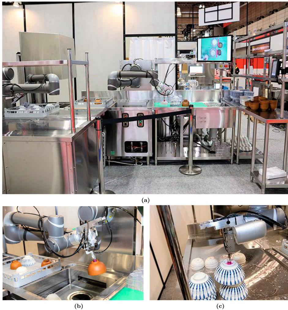
Figure 2. Commercial dishwasher system robot setup. (a) Dishwasher system robot setup. (b) Pick and pre-wash dishes before placing them on the rack. (c) Sort and place the washed dishes.
